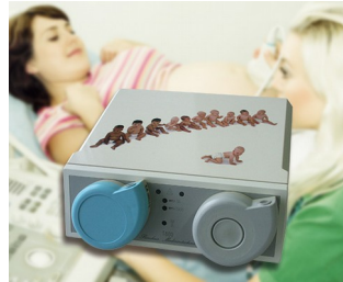
Telemetry system with cordless sensors
