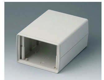
A9413440 SHELL-TYPE CASES O 190, Vers. I ABS (UL 94 HB) off-white RAL 9002 138x190x91mm
