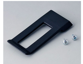
A9172109 Belt/Pocket clip ABS (UL 94 HB) black RAL 9005 62x30mm
