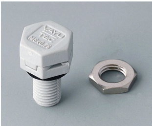
C2306917 Pressure equalisation element M6x0.75 PA 6 (UL 94 HB) light grey RAL 7035
