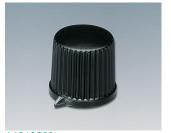
A1312560 TUNING KNOB, with lateral screw fixing ABS (UL 94 HB) black RAL 9005 20.7x19.7mm 6mm
