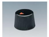
A1316240 TUNING KNOB, with lateral screw fixing ABS (UL 94 HB) black RAL 9005 16.4x12.3mm 4mm
