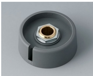
A3040088 COM-KNOBS 40, with recess PA 6 volcano 40x16mm 8mm
