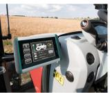
ISOBUS terminal for tractors and self-propelled machines
