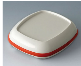
B1606207 BODY-CASE L, with recess ASA (UL 94 HB) traffic white RAL 9016 55x46x17mm IP 65
