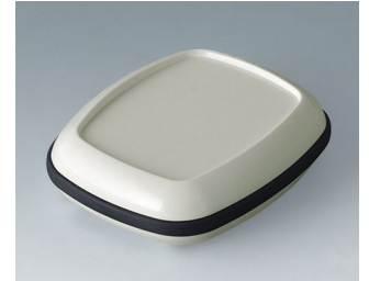
B1604217 BODY-CASE M, with recess ASA (UL 94 HB) traffic white RAL 9016 50x41x16mm IP 65
