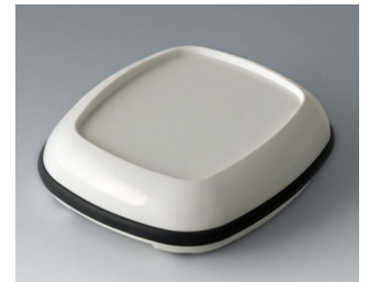
B1606217 BODY-CASE L, with recess ASA (UL 94 HB) traffic white RAL 9016 55x46x17mm IP 65
