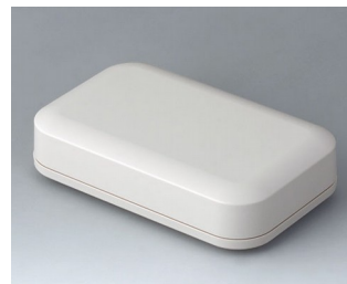
A9441107 EVOTEC 150, Vers. I ASA+PC-FR (UL 94 V-0) off-white RAL 9002 150x93x35mm IP 65 opt., IP 40
