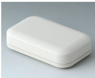
A9421107 EVOTEC 100, Vers. I ASA+PC-FR (UL 94 V-0) off-white RAL 9002 100x62x26mm IP 65 opt., IP 40
