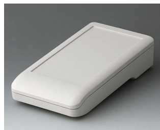
A9006117 DATEC-COMPACT M ASA+PC (UL 94 V-0) off-white RAL 9002 172x92x39mm IP 41
