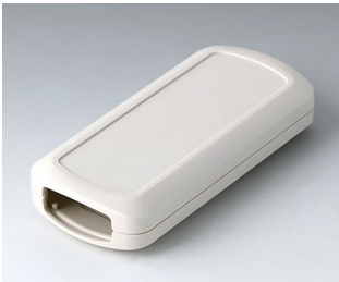
B2833107 CONNECT M ASA+PC (UL 94 V-0) off-white RAL 9002 116x54x22mm
