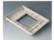
B4042717 Bottom part S flat, version II ABS (UL 94 HB) off-white RAL 9002 190x135x24.5mm IP 54 opt.
