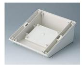
B4044827 Base M - desk-top -ABS (UL 94 HB) off-white RAL 9002 153x153x63mm
