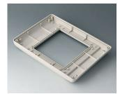
B4044707 Bottom part M flat, version I ABS (UL 94 HB) off-white RAL 9002 225x165x25.5mm IP 54 opt.
