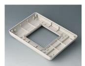
B4042707 Bottom part S flat, version I ABS (UL 94 HB) off-white RAL 9002 190x135x24.5mm IP 54 opt.
