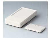
A9072127 DATEC-POCKET-BOX L ABS (UL 94 HB) off-white RAL 9002 120x65x22mm IP 41
